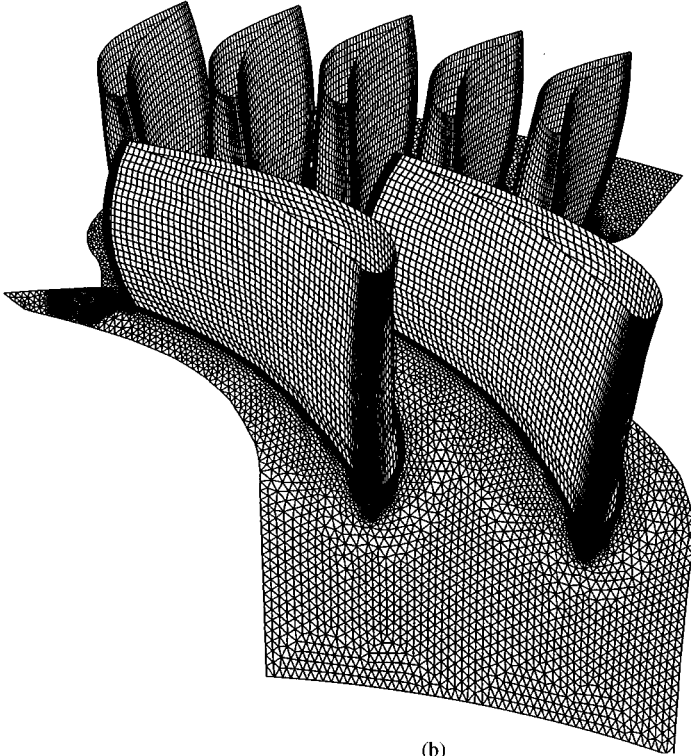
Figure 5. (a) Viscous and inviscid meshes for a typical sector (rotor mesh is inviscid in both cases), and (b) 3-D view of the rotor/stator mesh.
