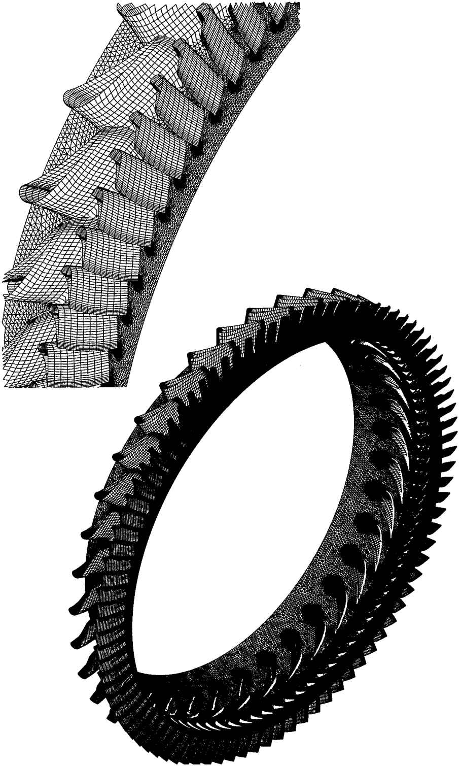
Figure 12. Multi-stage whole-annulus model for low-engine-order calculations.
